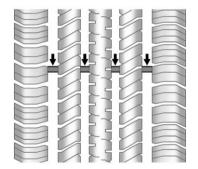
One way to tell when it is time for new tires is to check the treadwear indicators, which appear when the tires have only 1.6 mm (1/16 in) or less of tread remaining. See *Tire Inspection on page 10-50* and *Tire Rotation on page 10-50* for additional information.
